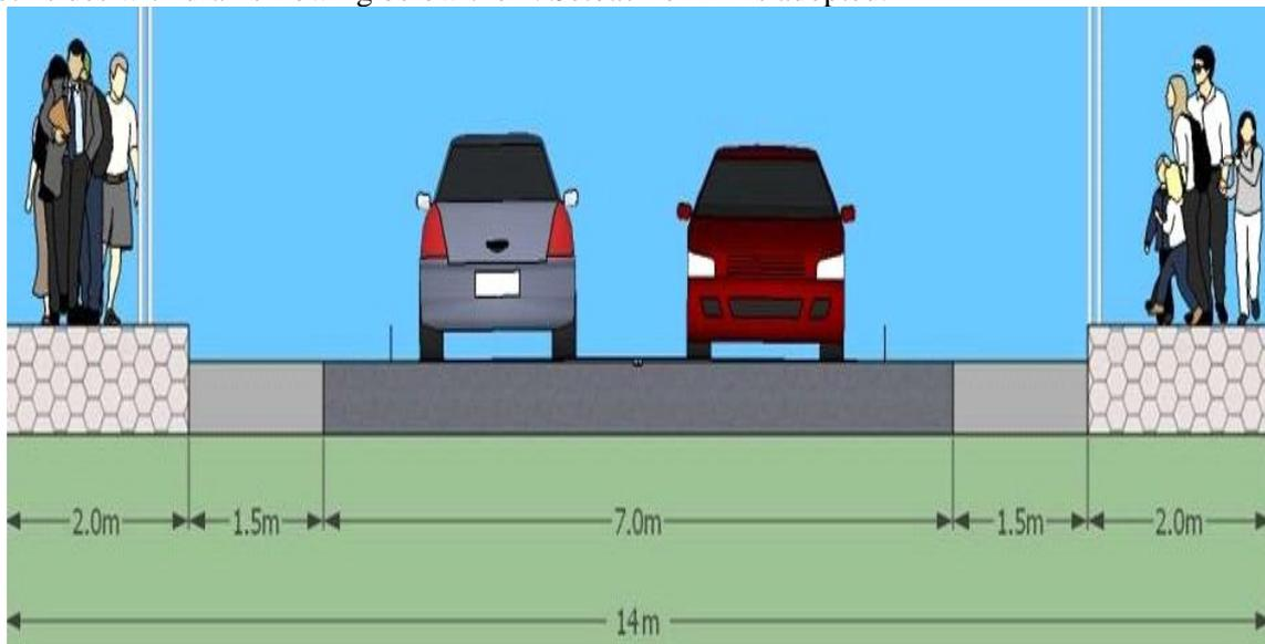
**Fig. 4:** Typical Cross section of A Class Road
