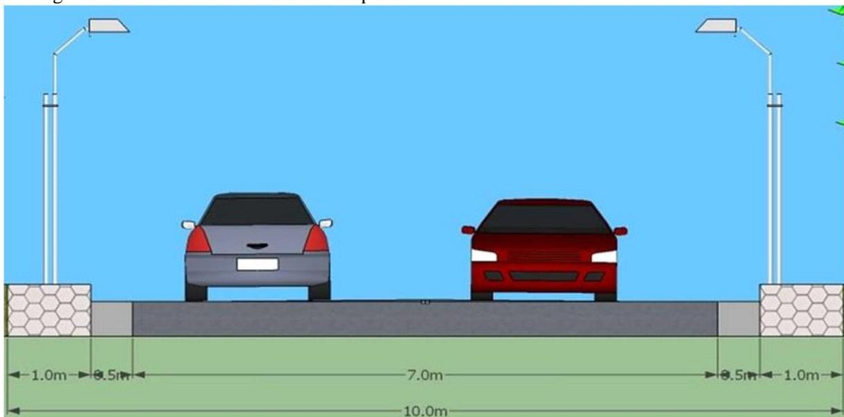
Fig. 5: Typical cross section of Ring Road
